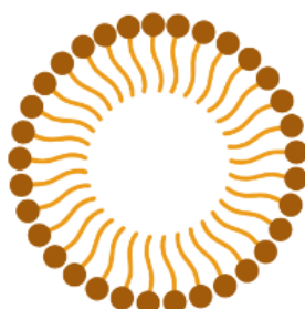
Figure 2.5: Schematic illustration of a spherical micelle. This illustration shows the configuration of a spherical micelle aggregate with the hydrophilic 'head groups' orientated towards the aqueous phase on the outside, limiting the contact between the hydrophobic 'tail groups' and the water. Created with BioRender.com
